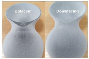
Figure 22: Orientation of features
