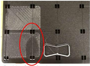
Residue from first layer is not present where oils are on substrate (indication of low adhesion). Normal handling typically leads to a build up of oil near edges and corners of substrate. This will lead to low adhesion for parts built in those areas.
