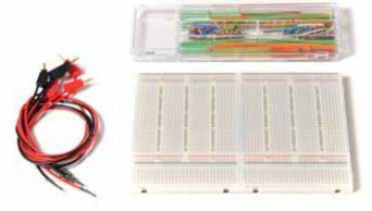
Breadboard for circuit configuration with wired components
