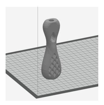
Flat surfaces positioned at shallow angles often have aesthetic issues due to layer lines. To minimize these, the surface can either be faced downwards or it can be rotated to a greater angle from horizontal, this will increase the number of layer lines on the surface and provide a more uniform appearance.
