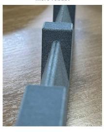
The same effect can also be observed on square edges of up facing material. The slight meniscus lip around the edge can become damaged and look untidy, Figure 6. Adding a very small radius (1mm) to these square edges can mitigate the lipping and reduce damage during depowdering. This approach avoids having to reorient the part in the nest which could compromise aesthetics.
