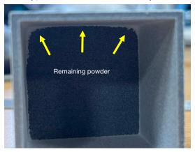
With a radius applied, powder is easily removed
