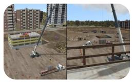
Signal Person Views A fixed view of the lift area, with the crane, load and target visible. A dynamic view that follows the movement of the load.
