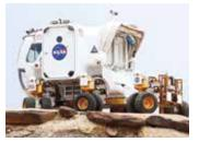
This rover, which has a pressurized cabin to support astronauts, includes about 70 FDM parts, including housings, vents and fixtures.
