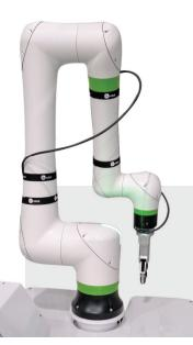
Adding to CRX Application flexibility is FANUC force sensors. A force sensor gives the robot the sense of touch and feel. This is very useful for material removal, including sanding, buffing, and deburring, as well as assembly applications. Force sensors are plug and play with FANUC's cobots including the CRX.
