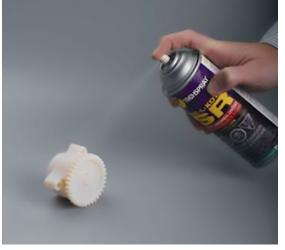
Figure 1. Applying chemical resistance spray on assembled parts.
