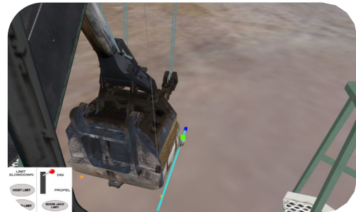
Controlling the dipper by following a straight-line trajectory
